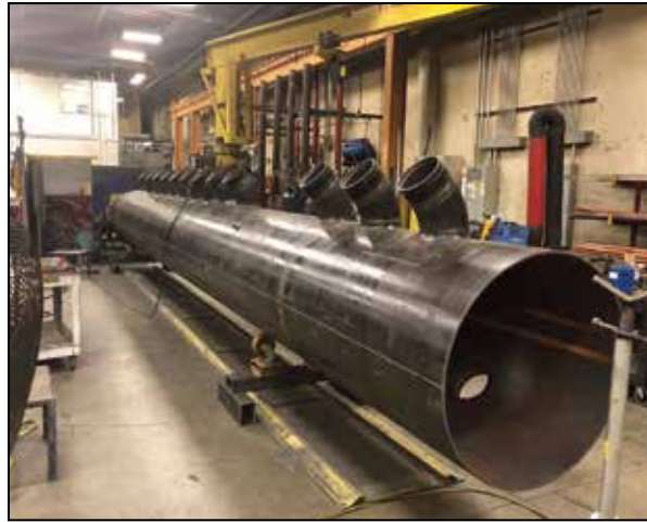
A 54 Compressed Air Header built in the shop for a Boeing project for MacMiller.
