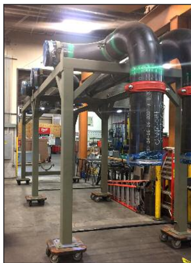
Prefabricated pipe rack built in MacDonald Miller's Fab Shop destined for Oregon job.
