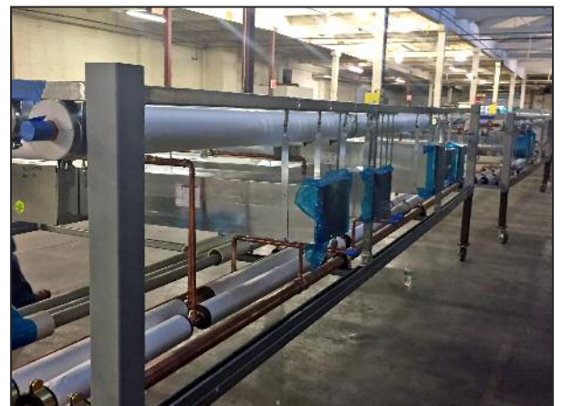
Trade rack—Prefabricated trade rack in McKinstry's fab shop destined for UW Medicine 3.2"
