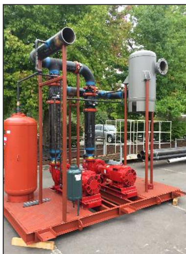
Pump skid built at PSF Mechanical's fab shop destined for 1005 Broadway job.
